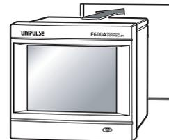
4. Install from the rear the guide rails having been removed from both sides in Step 2, and fix them with the screws (two).
